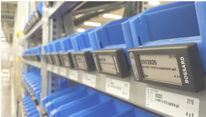
SmartLabel is an intelligent label which can be fixed on every possible storage bin. It displays all relevant product information as well as real-time order status and delivery date. Users can also release orders directly at the point of use at the touch of a button. The SmartLabel display is based on e-paper technology. It is easy to read under all lighting conditions and a long battery life ensures minimal maintenance.
